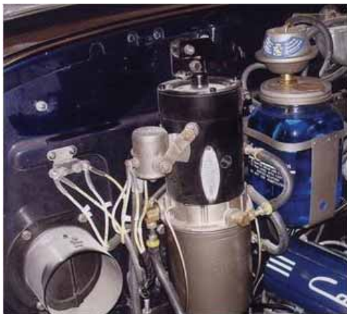
1949 HYDRO-LECTRIC PUMP (Ventilating tube removed for clarity.)
